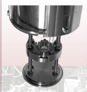
The reactor Chamber can be equipped customized with various sample holder receiving stations (flag style, Cameca, OmniVac). Internal shielding prevents the Chamber and windows from excessive heat. Flanges for sample transfer, viewports etc. can be customized optionally a gas mixing station for controlled inlet of up to 4 gases via MFCs can be provided.
