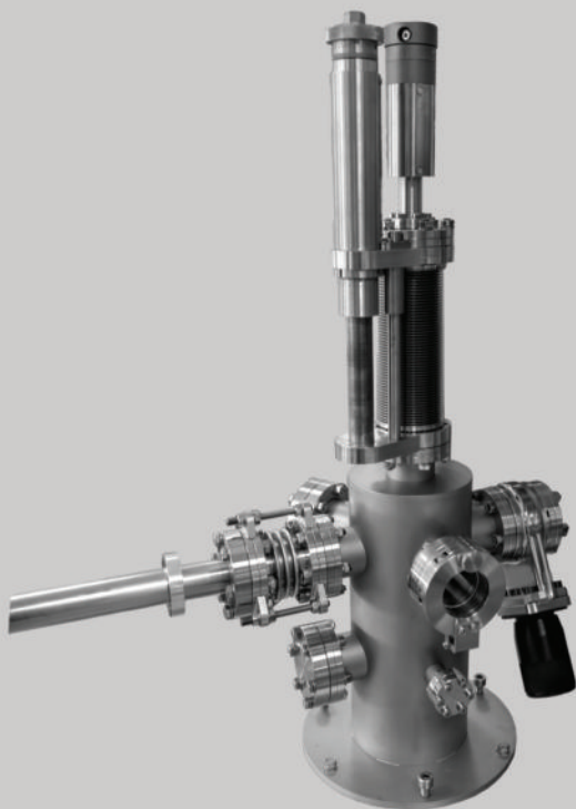
Load lock chamber with sample storage and transfer
